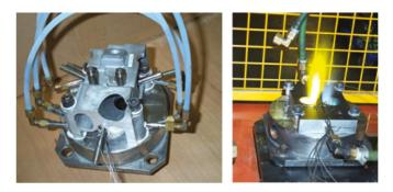
Figure 14. Single-cylinder specimens and experimental set-up with blowtorch heating.
