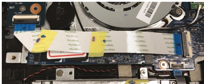
Figure 4. Poor design of overlapping of soft wiring and Solid-state drive.
