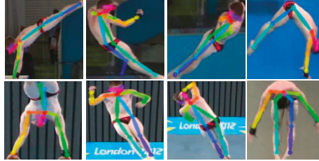
Figure 5. Joint trajectories of two different views for the same person performing diving. (The first row shows results on the side view and the second row presents results on the front view.).
