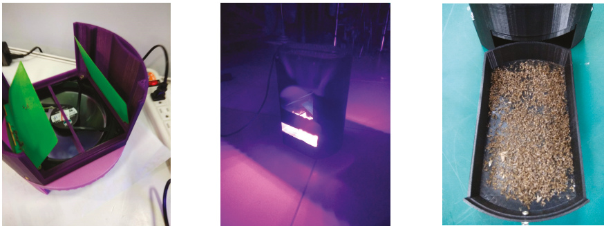
Figure 7. Proposed mosquito trapper with Secondary Freeform Lens Device and its mosquito trapping results.
