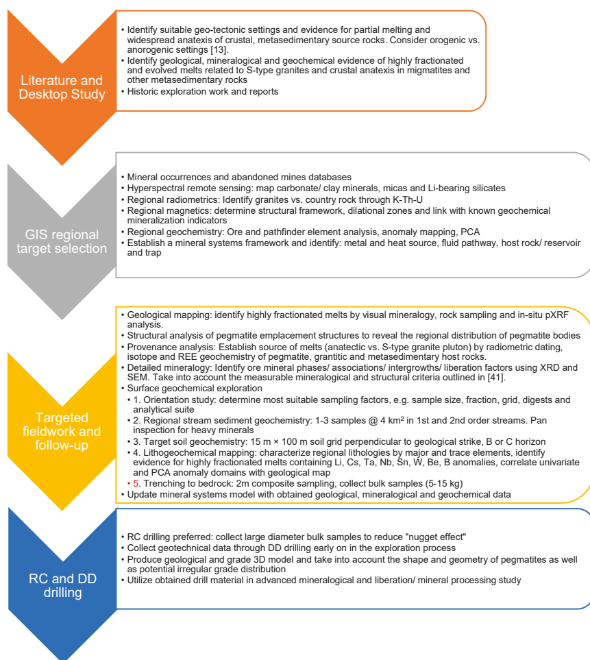
Figure 4. Workflow for early-stage LCT pegmatite target generation, definition and testing.
