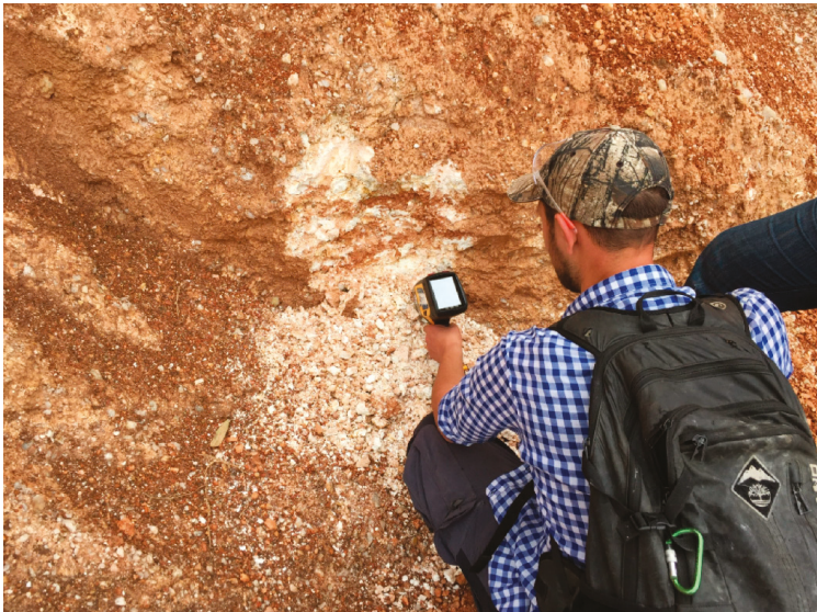
Figure 5. Portable XRF (pXRF) equipment is a valuable screening tool in grassroots LCT pegmatite exploration. At Ruhanga (Rwanda), B horizon soils overlying kaolinised LCT pegmatite contained large flakes of muscovite. Analysis by pXRF provided K/Rb values of 4.8, indicating highly fractionated bedrock and therefore a possible target [45].
