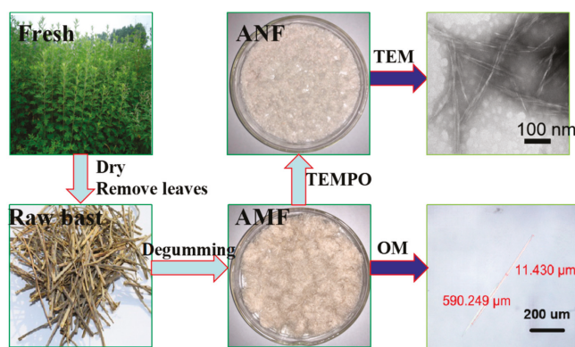
Figure 1. Flowchart of the Artemisia vulgaris bast microcellulose fiber (AMF) and Artemisia vulgaris bast nanocellulose fiber (ANF) extraction. (TEM, transmission electron microscopy. OM, optical microscopy. TEMPO, 2,2, 6,6-tetramethylpiperidine-1-oxyl).
