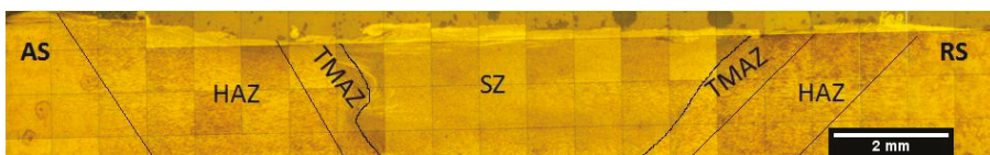
Figure 3. Friction stir welding micro-structural zones.
