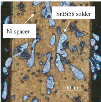
Figure 7. The laminated ACFs on the PCB electroless nickel immersion gold (ENIG) metal electrodes.
