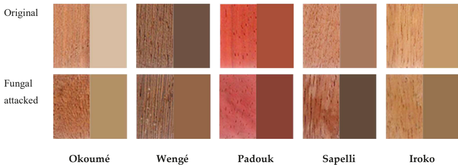
Figure 3. Visualization and pantone swatches of the top surfaces of selected tropical woods before and after exposure to C. puteana .
