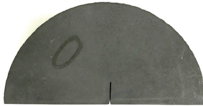
Figure 1. Notched semi-circular bend (NSCB) sample.
