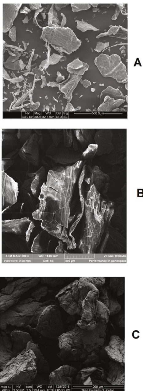
Figure 1. SEM images of raw chitin (A), ball milled chitin (B), and compacted chitin (C).
