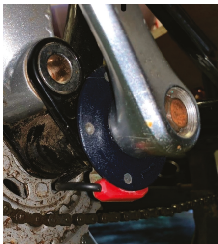
Figure 15. Cadence sensor assembly.
