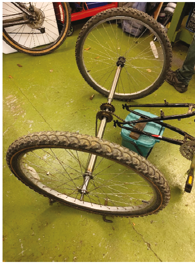
Figure 11. Rear shaft and axle assembly.
