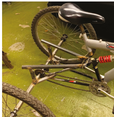
Figure 12. Platform frame assembly.
