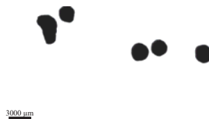
Figure 1. Shadows of granules digital images were captured with a linear video camera.
