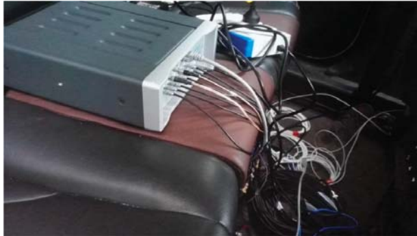
Figure 15. Digital acquisition hardware inside the car.
