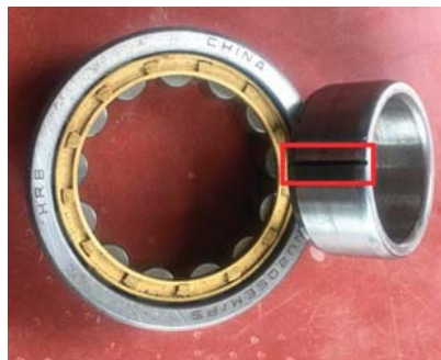
Figure 2. The inner race fault of the roller bearing.
