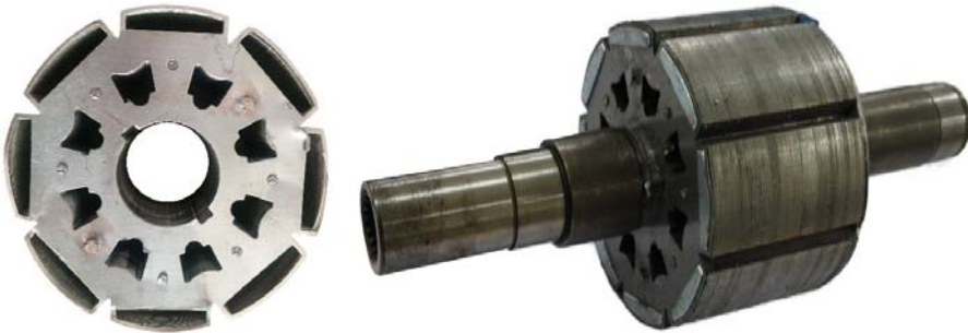
Figure 7. The rotor structure of the novel SIPMSM.
