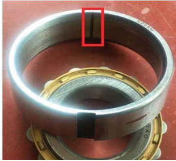
Figure 3. The outer race fault of the roller bearing.
