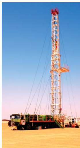
Figure 1. Mobile oil drilling plant type TW125 CAA6 mounted on a chassis ROMAN 75,540 MFEG (12 × 8) [24].
