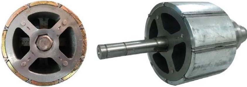
Figure 6. The rotor structure of traditional SIPMSM.
