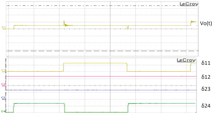
Figure 21. Output voltage V_o(t) and switching patterns sent to T11, T12, T23, and T24 (ZOOM 1 in Figure 20).
