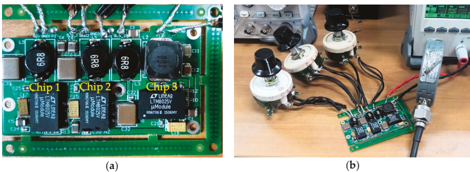
Figure 16. Photos of the power supply module instance. (a) PCB and its layouts; (b) Experimental scenario.
