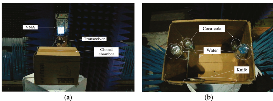
Figure 18. Imaging test for closed chamber. (a) Imaging system and target scene; (b) distribution of targets.
