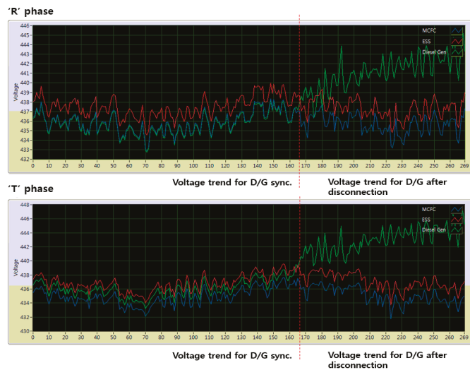
Figure 22. Voltage change when diesel generators are broken away.
