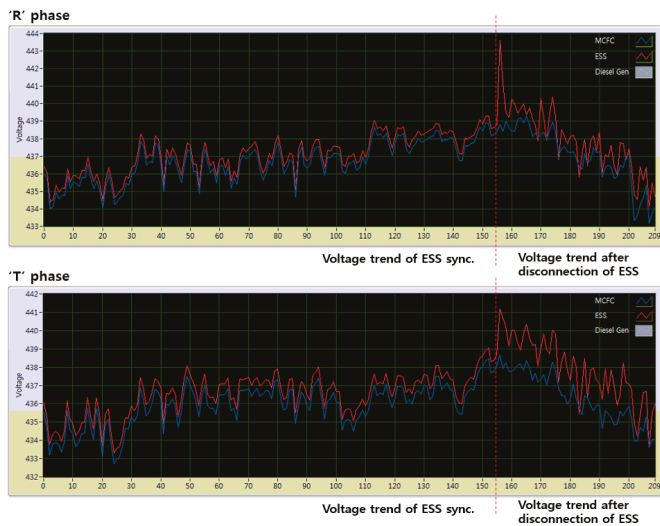
Figure 18. Voltage change when the ESS system was disconnected.
