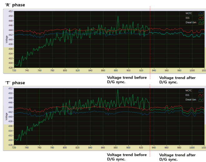
Figure 20. Voltage change when synchronizing diesel generators.
