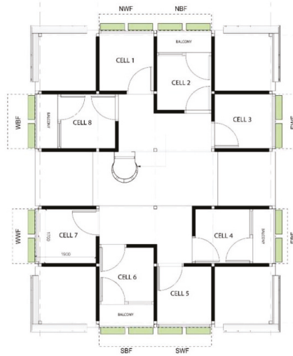
Figure 2. Floor plan of the Tropical Technologies Laboratory (T 2 Lab) indicating the eight test bed cells and facades analyzed in this study. Adapted from: AWP Architects based on lead author’s preliminary design.
