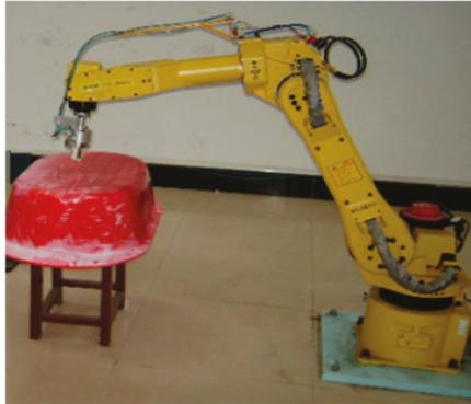
Figure 13. Spray painting Experiment in the Laboratory.
