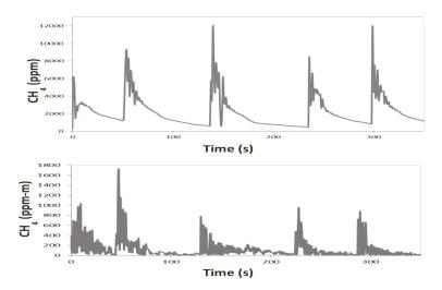
**Figure 1.** Representation of CH<sub>4</sub> concentration for a cow measured with a non-dispersive infrared (NDIR) sensor (above), and laser methane detector (LMD; below) with different belching events.
