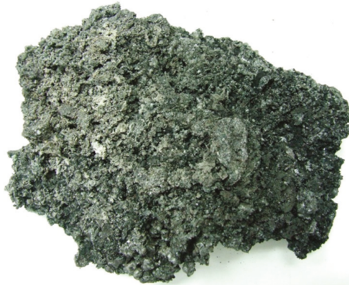
Figure 5. Incrust from the grate section of generator.
