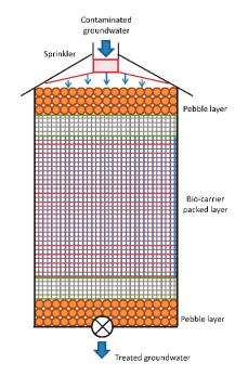
Figure 7. Configuration of the pilot plant feasibility test. Adapted from [39,46].
