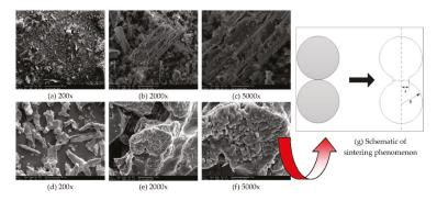
Figure 3. SEM images of rice straw ash at 400 °C (a-c) and 800 °C (d-f) and schematic of sintering phenomenon (g).
