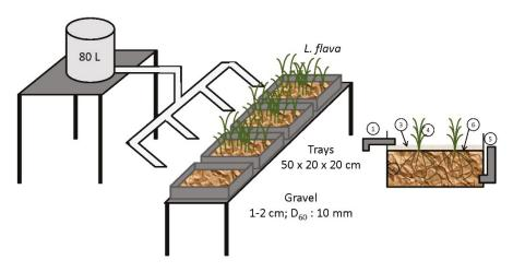
**Figure 8.** Schematic view of experimental setup in the pilot-scale constructed wetland system. Lateral section of planted systems *Limnocharis flava*: 1. Supply pipe; 2. Distribution area (coarse gravel); 3. Gravel 1-2 cm; D60: 10 mm; 4. *Limnocharis flava*; 5. Adjustable output pipe to control water level; 6. Water level. Adapted from [68].
