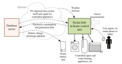
Figure 2. CEGADS system diagram.
