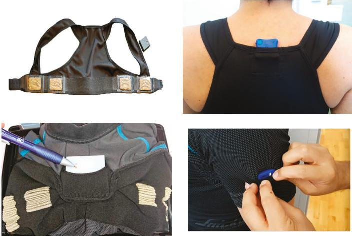
Figure 2. Vest (top) and t-shirt (bottom), including textrodes and ECGZ2 and IMUs.
