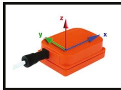
Figure 5. The Xsens MTx unit [44].
