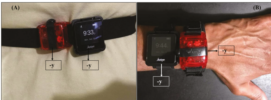
Figure 5. Orientation of the axes in the GT3X+ and GT9X when worn on the hip (A) and wrist (B), respectively.
