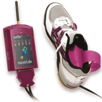
Figure 6. Foot-pressure monitoring system, Pedar (Novel, Munich, Germany, www.novel.de ).
