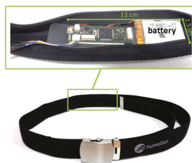
Figure 4. The sensor belt includes a 3D accelerometer, gyroscope and magnetometer, as well as a barometer.
