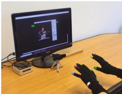
Figure 1. System for the upper limbs analysis: RGB-Depth camera (Intel RealSense ® SR300); NUC i7 Intel ® mini-PC; lightweight gloves with color markers.
