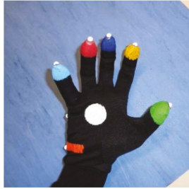
Figure 4. HCI glove with reflective markers on the finger tips.
