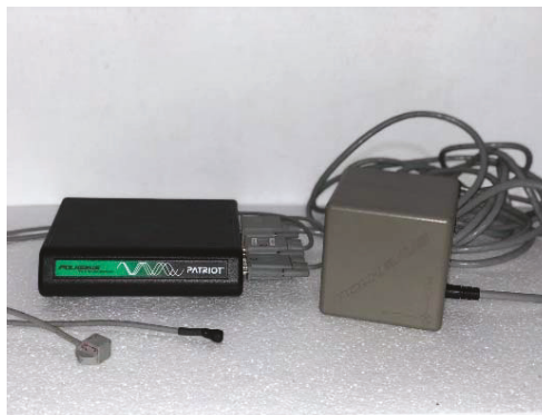
Figure 1. Polhemus device. From left to the right: sensors, receiver module, emitter module.
