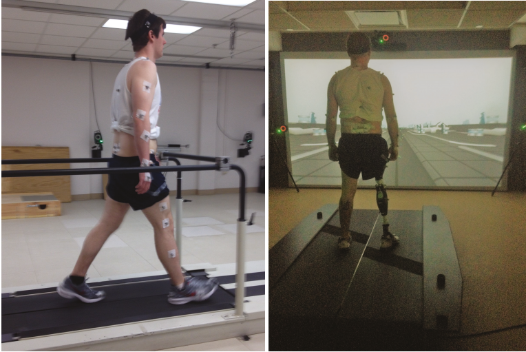
Figure 2. Experimental setup for data collection. The left figure shows an able-bodied subject and the right figure shows an amputee subject with an Ottobock prosthesis on the right leg.
