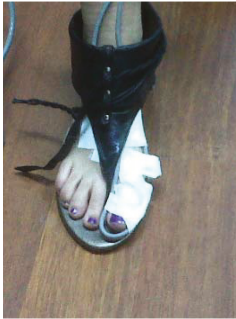
Figure 4. Fastening of the sensors. White bandages are auto-adhesive fixatives.
