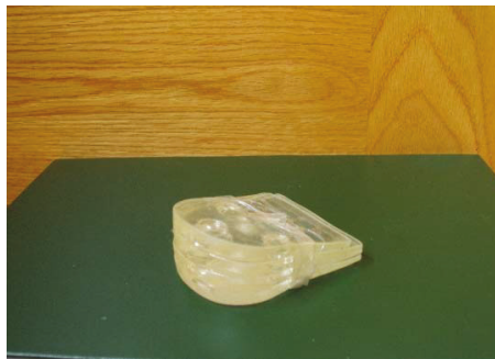
Figure 6. Prefabricated high-heels. The heels were made on hard silicone. The additional height was added over the top.
