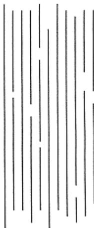
**Figure 1.** Ideal polymer chains model for producing high strength and high modulus fibers.
