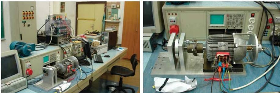
Figure 4. Experimental set-up for testing rotary synchronous machines at locked rotor.
