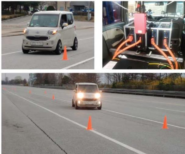
Figure 17. Slalom test and measuring sensor.
