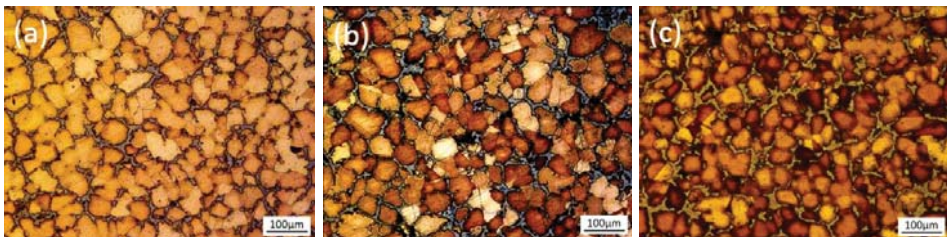
Figure 7. Microstructures of ZCuSn10P1 alloy at different pouring lengths at a pouring temperature of 1080 °C: (a) 200 mm; (b) 300 mm; and (c) 400 mm.
