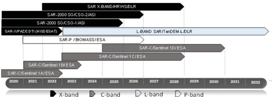
Figure 2. Frequency bands of future (2020–2030) European Union (EU) mission carrying Synthetic Aperture Radar (SAR) imager instruments.
