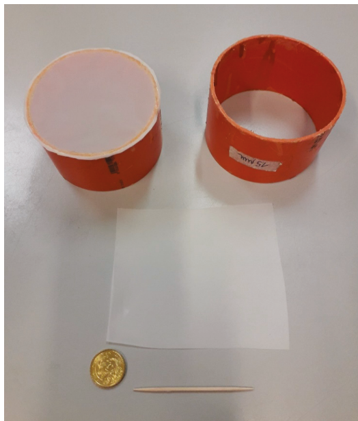
Figure 1. Tissue sieve made with nylon mesh. From bottom to top: toothpick and 100-cm 2 -piece of nylon mesh; PVC ring and tissue sieve ready for use.
