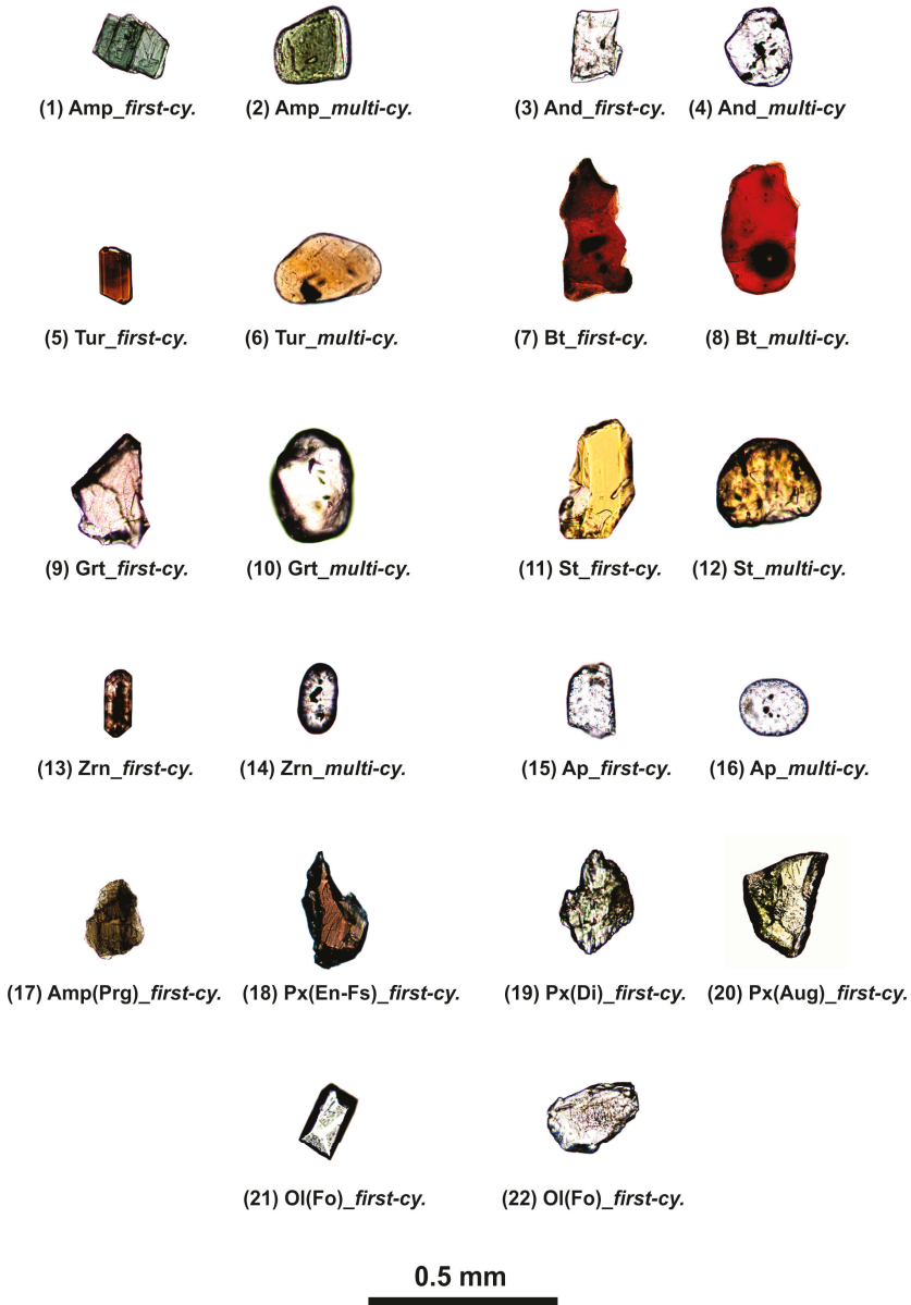
Figure 19. Typical visual aspects of the main heavy mineral transparent suite according to their dominant surface texture. Mineral grains classified with first-cy. are “first-cycle” particles that have angular to sub-angular surface textures and are catalogued with odd numbers from 1–15 and continuously from 17–22. In this class it was detected the presence of several euhedral Fo minerals (grain 21). Mineral grains classified with multi-cy. (catalogued with odd numbers from 2–16) correspond to the “multi-cycle” ones.
