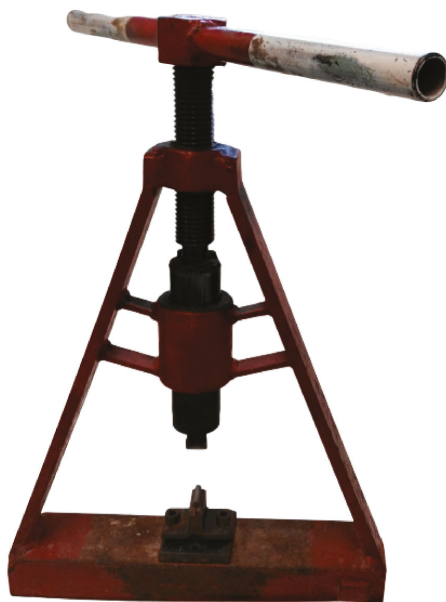
Figure 2. Manual press designed to split sedimentary rocks using protective eye goggles.
