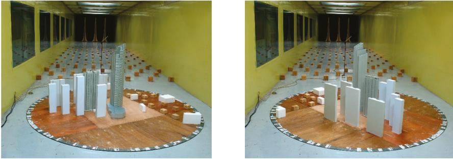
**Figure 4.** The rigid building model with existing surrounding conditions mounted in the wind tunnel lab of Shantou University from two different perspectives.
