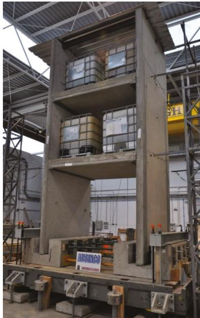
Figure 12. General view of the real-scale three-storey precast concrete building.
