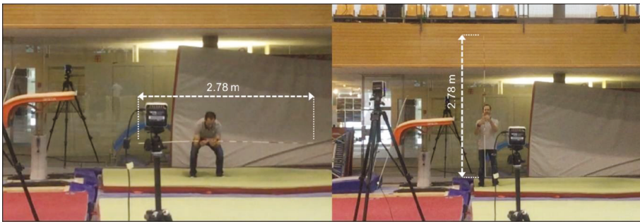
Figure 1. 2D calibration: calibration of measuring range by definition of reference height and width with the calibration rod (2.78 m) in the 2D-video software Dartfish (Dartfish SA, Fribourg, CH).
