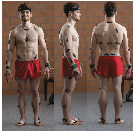
Figure 4. Plug-in Gait model: positioning of 43 markers for 3D analysis, attached to the athlete according to Vicon Plug-in Gait model [10].
