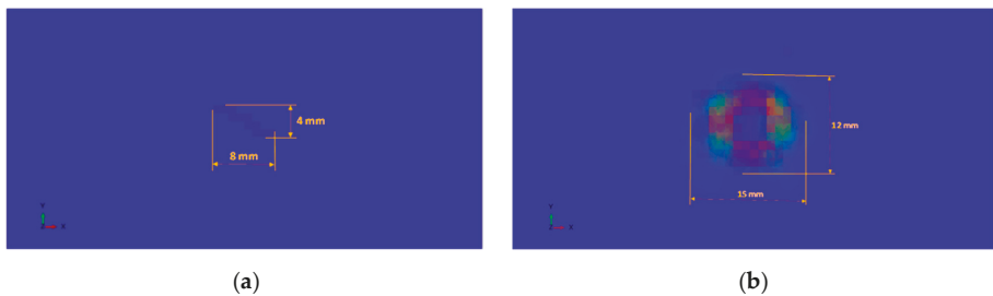
Figure 25. (a) Fiber compressive damage; (b) matrix tensile damage.
