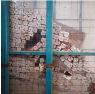
(a) Deformation after mining ore body #3
