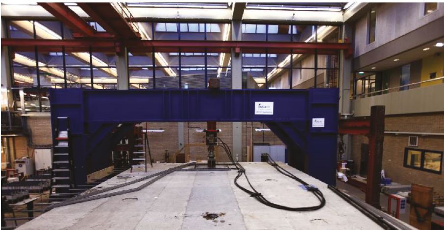
Figure 5. Overview of the test setup, showing setup 1 with the new middle deck.
