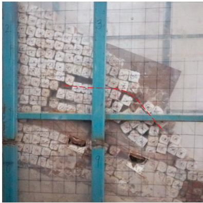
(a) Deformation after mining ore body #2
