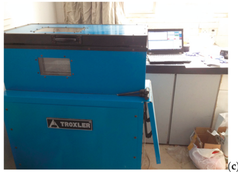
Figure 1. Three fatigue testing apparatuses: (a) four-point beam (4PB) fatigue test, (b) two-point trapezoidal beam test (Trapezoidal Beam), and (c) Overlay Tester.
