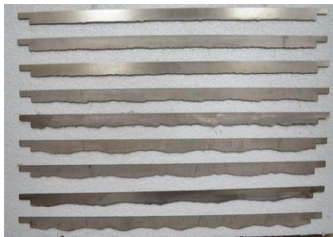
Figure 4. Steel sheets with Bardon's roughness profiles.
