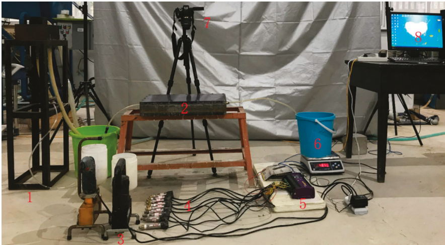
Figure 6. Picture of the experimental device. 1—Stable water head system; 2—the simulated fracture; 3—grouting pump; 4—pore pressure transducers; 5—data acquisition instrument; 6—weighing system; 7—image acquisition system; 8—computer.
