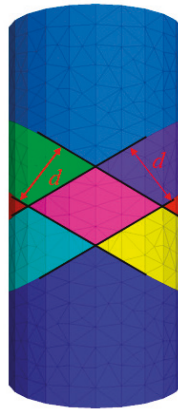
Figure 12. Rock specimen model with two intersection joints sets .
