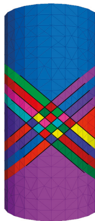
Figure 14. Rock specimen model with intersecting joints.
