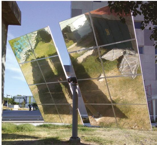
**Figure 18.** Heliostat.
