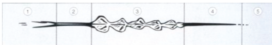
Figure 19. The different stages of dry time as determined visually versus time. Stage 5 is considered dry.
