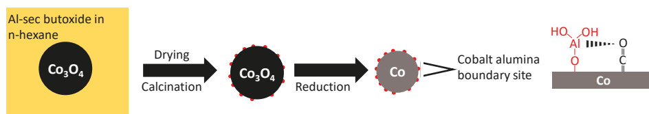
Figure 6. Schematic depiction of the formation of sub-nanometer-sized alumina islands upon impregnating a cobalt oxide surface with Al-sec butoxide in n-hexane, and their interaction with CO adsorbed on the reduced metal surface.
