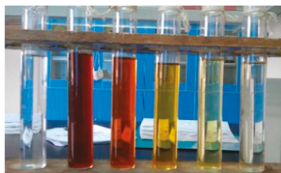
Figure 10. Effluent of catalytic-biological treatment portion (at 90th day). (Left to right: pure water/initial water/CBR-1/CBR-2/BAF-1/BAF-2).
