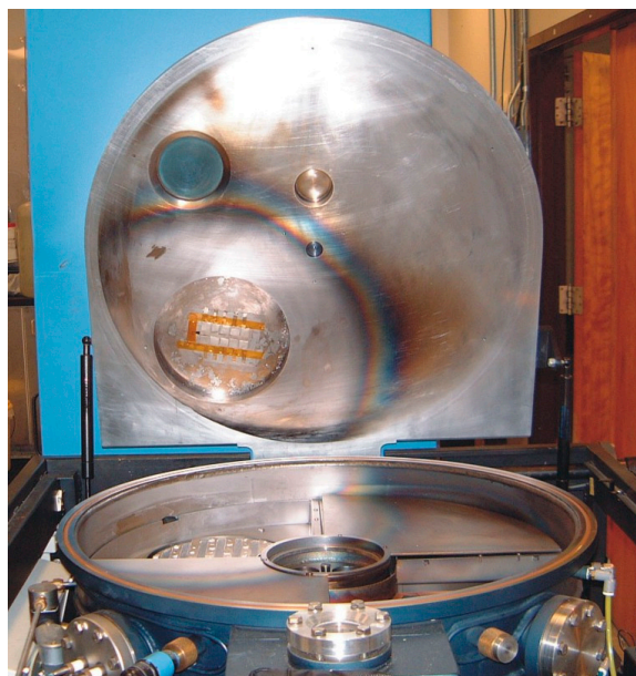
Figure 1. An radio frequency (RF)-sputtering unit with an 8" nickel target decorated with different amounts of modifying elements ( bottom ) and an array of sandblasted nickel substrates with silicon witness substrates for composition measurements ( top ). The substrates are taped to a copper plate with circulating ice water or liquid nitrogen.
