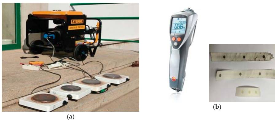
Figure 12. (a) Electrogenerator AYERBE, 5KVA, 230v tipo AY4000MN, heating plates of 1000 watts of power each and voltmeter-ammeter devise (yellow colour, on the floor); (b) TESTO 308 opacity meter, which operates as established by ASTM D 2156-94, Standard Test Method for Smoke Density in Flue Gases from Burning Distillate Fuels.
