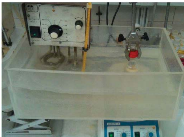
Figure 11. Experimental dispositive for the transesterification reaction.
