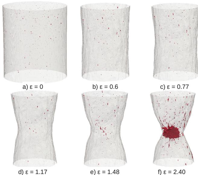
**Figure 3.** Damage evolution in the non-charged AISI316L sample observed as a volume rendering. The outer surface of the sample is transparent grey and the cavities are the dark red dots. Damage nucleates then grows and finally coalesce in the bottom right image (a) initial state; (b) true strain  $\epsilon = 0.6$ ; (c)  $\epsilon = 0.77$ ; (d)  $\epsilon = 1.17$ ; (e)  $\epsilon = 1.48$ ; (f)  $\epsilon = 2.40$ .
