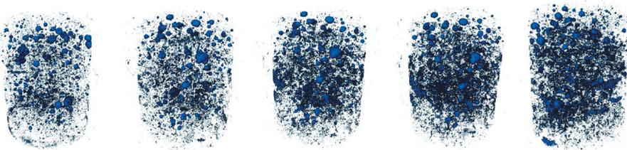
Figure 6. 3D views of the voids belonging to steel fiber-reinforced concrete at different ages. Age increases from left to right.
