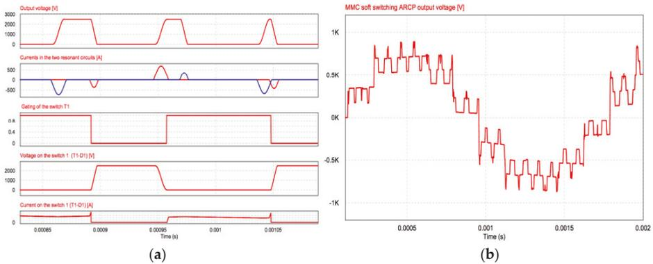
**Figure 12.** (a) Full H-bridge ARCP single submodule simulation diagram: output voltage, currents in the resonant circuits, gating of switch  $T_1$ , voltage on the switch 1, current on the switch 1. (b) Output voltage of a full ARCP soft-switching MMC (4-submodules for branch, all ARCP). Note: current and voltage values are scaled, for testing only.
