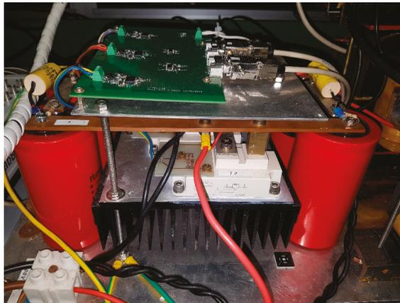
Figure 11. Converter prototype.
