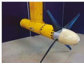
**Figure 1.** Tidal Turbine Testing (TTT) device and rotor.
