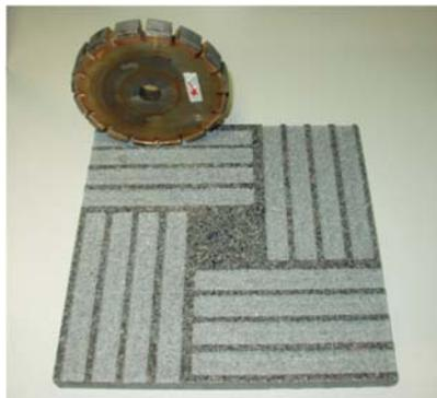
**Figure 8.** Sixteen grinding slots or grooves in one side of an Azul Alpalhão granite tile.
