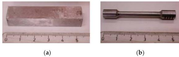
**Figure 2.** (a) Sintered body with dimensions of  $55 \times 11 \times 10 \text{ mm}^3$ ; (b) specimen used for tensile test.
