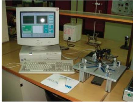
**Figure 5.** RFDA (Resonant Frequency and Damping Analyser) equipment (made by IMCE, Genk, Belgium) used for measuring the dynamic Young's modulus.
