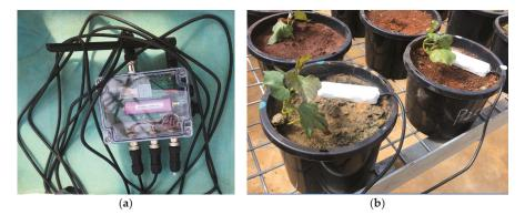
**Figure 2.** An example of a device with multiple sensors (**a**), with the ability to measure soil properties (**b**) (moisture, conductivity and temperature), air temperature and relative humidity. The device has a 2G/3G connectivity, and its web platform has an open Application Programming Interface (API) for ease of integration with other systems.
