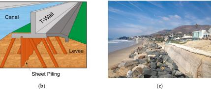
Figure 2. Types of flood protection: (a) a cross-section of a typical Dutch sea-dike, filled with sand and clay [14] (b) Two types of steel and concrete floodwalls applied [46] (c) Rip-rap [17].
