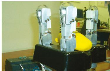
Figure 3. A prototype of LARM Hand IV.
