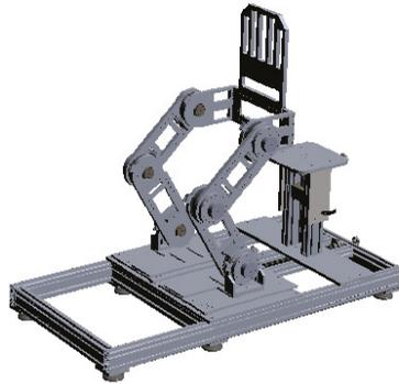
Figure 7. The prototype exoskeleton for the sit-to-stand exercise.
