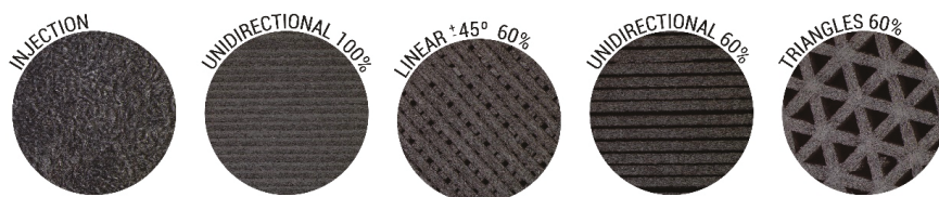
Figure 1. Stereomicroscope images ( \times 1.25 ) of the appearance of the injected and different patterned printed samples.
