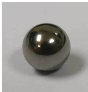
Figure 9. Steel sphere used in calibration.
