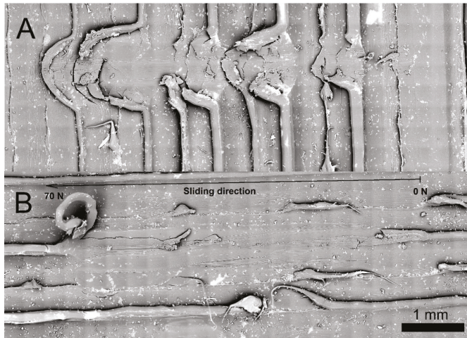
Figure 16. Micro scratch test: (A) perpendicular to the printing direction; (B) parallel to the printing direction.
