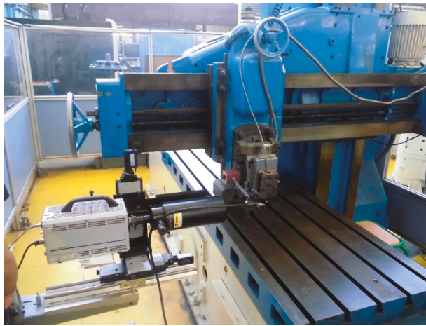
Figure 2. GSP 2108 R.20 shaping machine tool.
