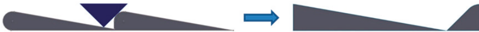
Figure 5. Representation of the roughness tip with the printed layers, for print orientation angle higher than 45^\circ .
