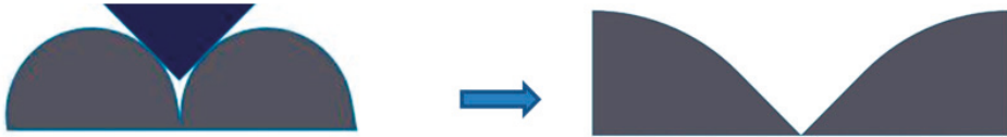
Figure 4. Schematic of the printed layers with the roughness tip, for print orientation angles higher than 45^\circ .
