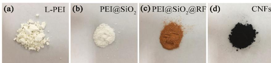
**Figure 2.** Photographs showing the evolution from linear PEI precursor to the CNFs during the synthesizing process. (a) Linear PEI, (b) PEI@SiO<sub>2</sub>, (c) PEI@SiO<sub>2</sub>@RF and (d) CNFs.
