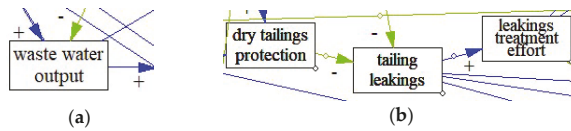
Figure 2. Elements in the CLD for the ITERAMS project (a) Example of state box: waste water output; (b) Example of relations described via arrows: tailings leaking.
