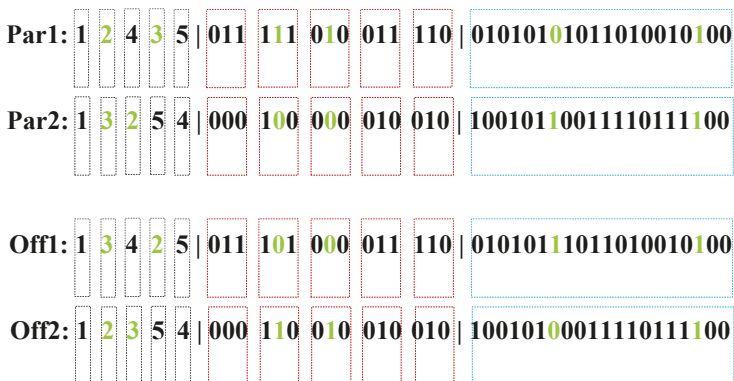
Figure 8. Two parent chromosomes and offspring after crossover operation.
