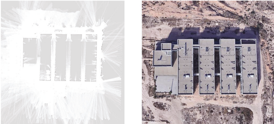
Figure 10. (left) Grid map of the secondary laboratory building, obtained using the architecture shown in Figure 2. (right) The actual building and the environment where the initial framework experiments have been carried out.
