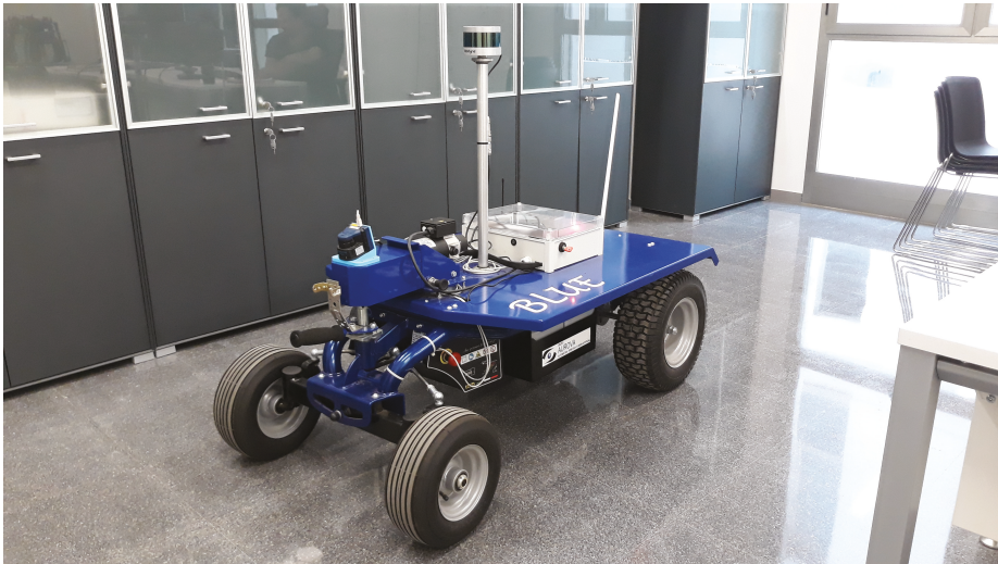
Figure 9. Experimental platform BLUE. This professional research platform—derived from a conventional electric cart—has been developed by our research group, in the University of Alicante. It is integrated with ROS and provides all the features required for developing state-of-the-art research in autonomous outdoor navigation.
