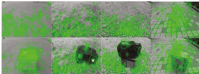
Figure 6. Distributions of feature points in terrain with and without obstacles.
