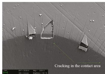
Figure 12. SEM observation of the indented surface of 2 µm CrN coated M50 disks under a load of 15 N and temperature of 500 °C.
