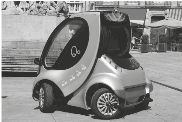
Figure 14. Hiriko Fold—a vehicle employing in-wheel motors.
