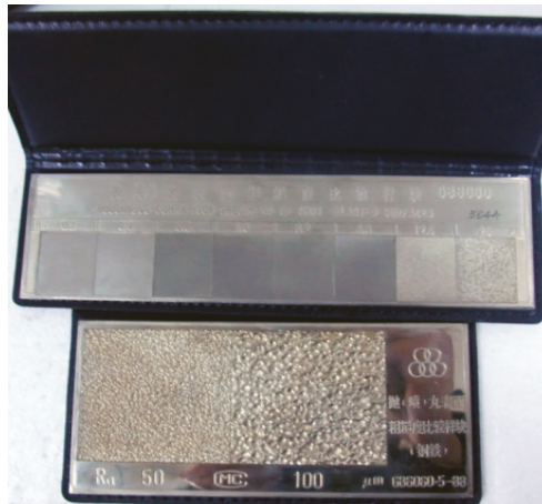
Figure 7. The samples with different surface roughness (material = SS).
