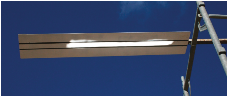
Figure 12. Concentrated radiation reflected into a Lambertian target.
