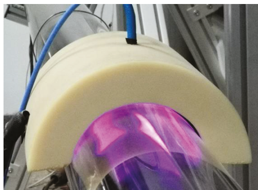
Figure 3. Emission image of air diffuse discharge at 700 Pa.
