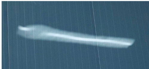
Figure 11. Reflected image for the assembly of naked mirror mechanically bended by metallic bars glued to it.
