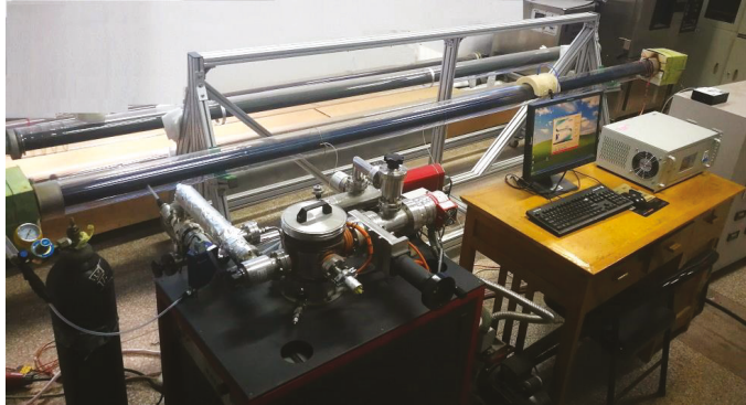
Figure 21. Residual gas analysis (RGA) system of the receiver.
