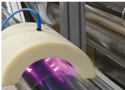
Figure 2. Emission image of air filamentous discharge at 7000 Pa.
