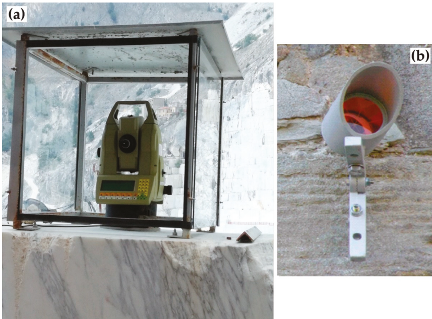
Figure 3. (a) RTS installed at the Lorano marble quarry. (b) Detail of a prism placed on the excavation site walls.
