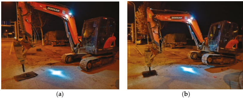
Figure 5. Two perturbation postures of the excavator: (a) fully and (b) partially touching the ground.
