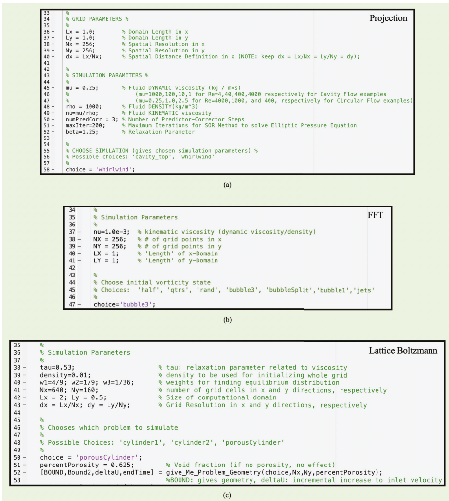
Figure 3. Options for practitioners to change the grid resolution and size, fluid properties (density, viscosity), and other solver attributes within the software for the (a) Projection method, (b) Fast Fourier Transform (FFT)-based spectral solver, and (c) Lattice Boltzmann solver. The possible choices for built-in examples are also listed for each.
