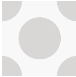
Figure 3. Representation of the material’s REV to be analyzed.
